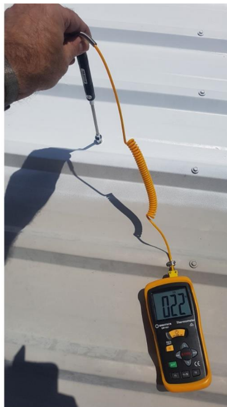
Roof temperature - surface sensor. Temperature measured with the surface probe. Surface covered with SFEROLIT coating
