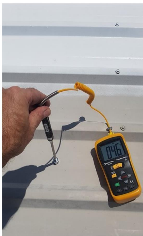
Roof temperature - surface sensor. Temperature measured with the surface probe. Surface covered with SFEROLIT coating
